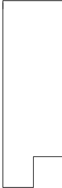
Figure 9.5.11: Definition region of the backward-facing step
