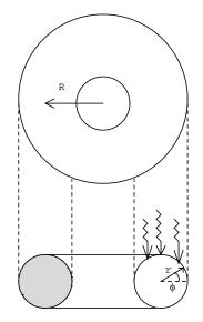
The sun shines on the toroidal object in the figure causing a heat flow into the object. The objective of this assignment is to calculate the thermal equilibrium in the object. Except for the solar radiation there are no heat sources.
