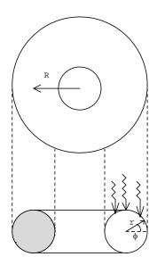
The sun shines on the toroidal object in the figure causing a heat flow into the object. The objective of this assignment is to calculate the thermal equilibrium in the object. Except for the solar radiation there are no heat sources.
