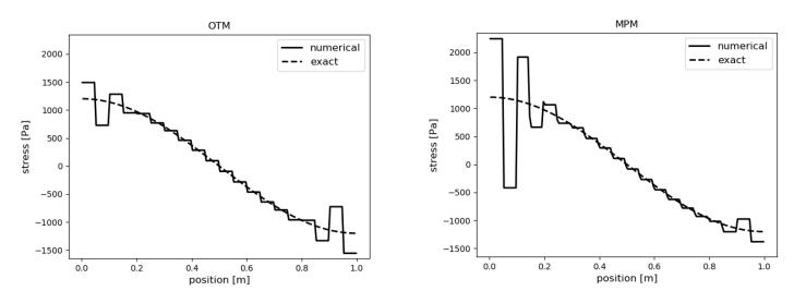
Figure 1 Comparison of numerical and analytical results in stress for OTM and MPM
