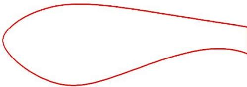
Current wind turbine rotor designs tend to employ very thick airfoil sections, possibly with very thick airfoil trailing edges. Combined with the nature of the flow in which wind turbines operate, this leads to unsteady flow features even in relatively benign flow conditions.
