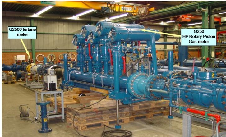
In order to realize traceability to international standards, every device that measures a certain property, e.g. meter per second, needs to be calibrated against the aforementioned international standards. Some flow meters, however, are used in a
