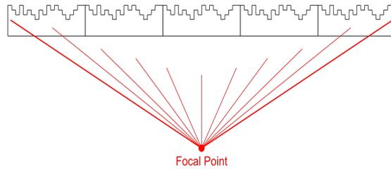
Figure 13: Far field design case. All lenslets focus on a single faraway point, meaning that now they must be not identical.
