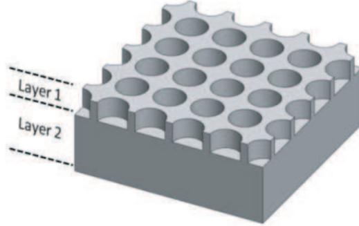
Figure 1: A layered, periodic dielectric structure.
