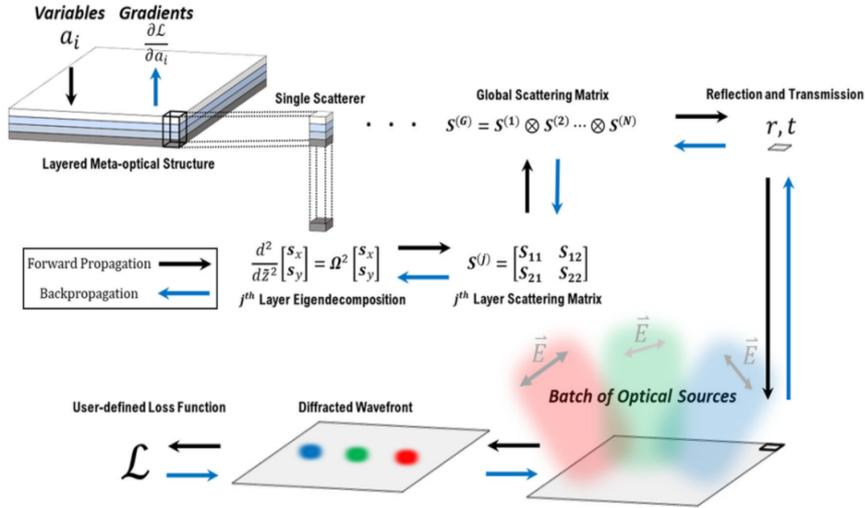
Figure 6: Colburn and Majumdar's scheme for metamaterial design with RCWA and algorithmic differentiation. The figure follows all notation I have used in my section on RCWA.
