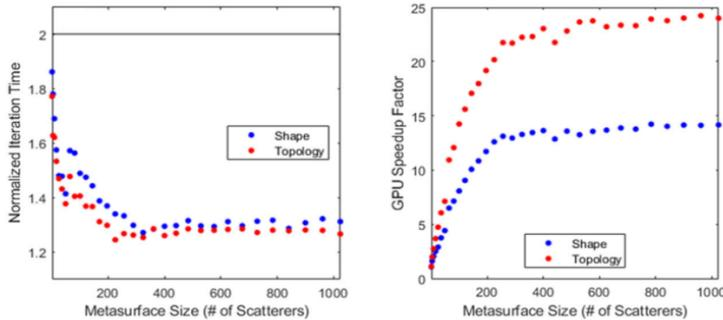
Figure 7: Performance results for the Colburn-Majumdar metaoptics optimization scheme. Both simple optimization of scatterer shape and full topology optimization are considered. Left: optimization iteration time, normalized to the time of a single forward simulation, are compared to the adjoint method (black horizontal line). Right: speedup factor from GPU parallelization vs. problem complexity.
