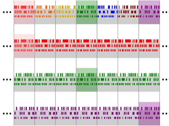
Figure 9: Lin et al. approximate the near field scattering pattern of an arbitrary aperiodic layered metasurface, shown at top, by solving a separate periodic scattering problem for each unit cell. These solutions, shown in the lower three rows, are combined to approximate the near field on the entire surface.
