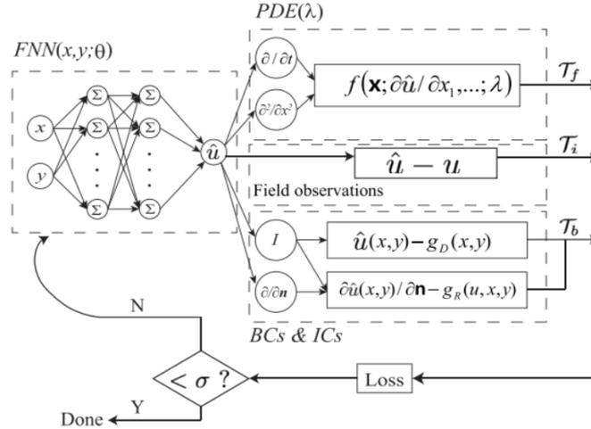
Figure 4: Framework of a general PINN, for the inverse problem to obtain PDE parameter  $\lambda$ . The left FNN (feed-forward neural network) is a model of the PDE solution, and the right side shows the terms of the loss function.
