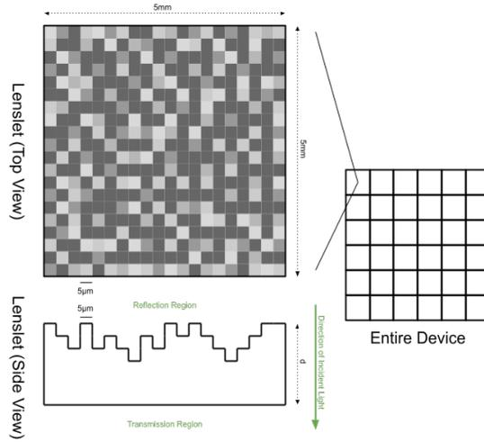
Figure 11: Basic proposed design of metasurface lens for COPILOT, consisting of an array of flat metasurface lenslets. This diagram shows 20x20 pixels per lenslet, which will in reality be 1000x1000. Lenslet thickness  $d$  and dimensions of lenslet array to be determined.
