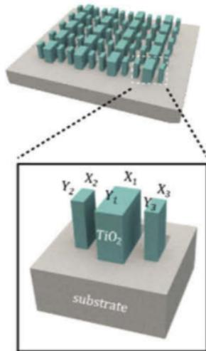
Figure 2: Metasurface design sought by Jiang et al. composed of repeating nanofin structures.
