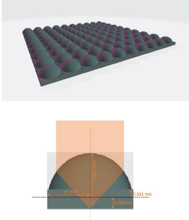
Figure 10: Existing lens design to be replaced, consisting of an array of traditional refractive lenslets.
