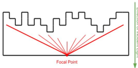
Figure 12: Near field design case. The focal point of each lenslet is the center of its transmission side surface, and all lenslets are identical.
