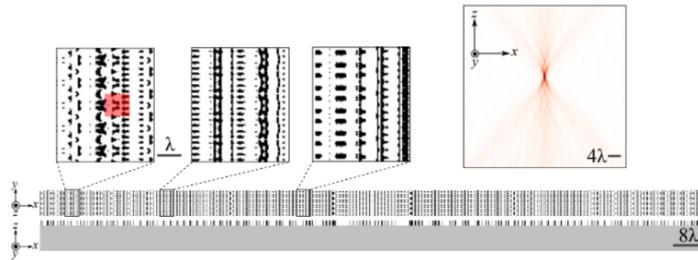
Figure 8: Monochromatic 3d cylindrical metalens topography achieved through adjoint method optimization by Lin et al. Red section shows a single  $\lambda \times \lambda$  unit cell. Plot on the right shows simulation of the final focusing behavior.
