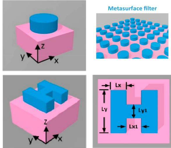
Figure 3: Metasurface design sought by An al. composed of arrays of dielectric "meta-atoms". Separate DNNs are employed for parameter selection of each meta-atom structure, such as the cylindrical and H-shaped ones seen here.
