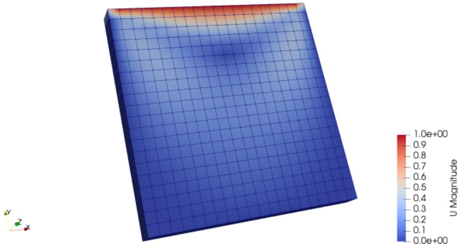
Left, right and down side of the square are walls, at the top the fluid is moved with velocity 1 in the right direction.
