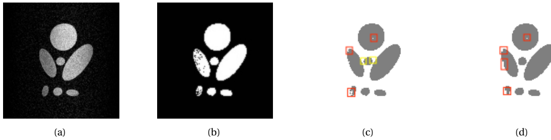
Figure 6.15: (a) Raw image. (b) Filtered image with the parameters d_p = 1, \eta = 10^5, K = 1 used. (c) Segmented image with the parameters n_{cl} = 1, n_b = 0 without HE. (d) Segmented image with the parameters n_{cl} = 1, n_b = 1 without HE.
