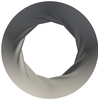
(c) Top view of the deformed annulus using the Kirchhoff-Love shell model.
