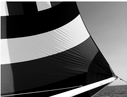
(a) Wrinkles in the corner of the spinnaker of the Andante , a classical example of wrinkling under in-plane loading.
