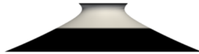
(b) Side view of the deformed annulus using the tension field theory membrane model. The black region denotes a taut, and the gray region denotes a wrinkled region.
