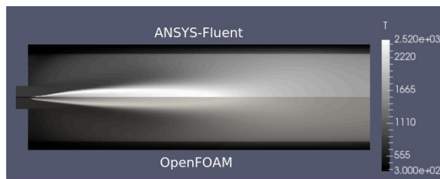
Figure 7: Comparison of the contour plots of the temperature (K) in Case 3 (radiation switched off).
