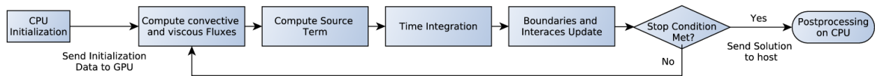
FIGURE 1. The Solver computes firsts inviscid and viscous Residuals and source term. Second the time integration takes places and finally boundaries and mesh interfaces are updated
