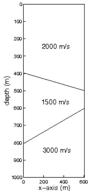
FIG. 1. Problem geometry with sound velocity profile.
