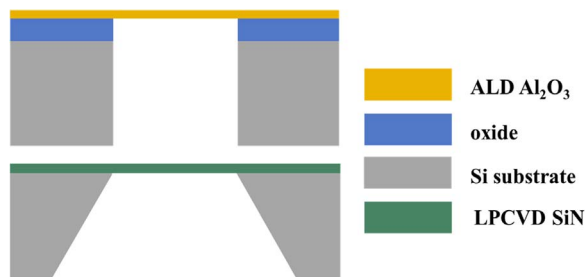
Fig. 12. Schematic (not to scale) drawing of suspended alumina (up) and SiN (below) single membranes fabricated for measurement of SEY.
