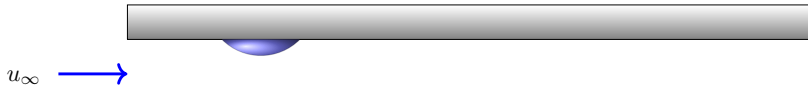
Figure 3: Basic setup of a single droplet attached to a flat surface, blown by an imposed free-stream airflow u_\infty .
