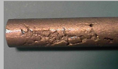
Preferential flow effect, one of the casting defects.
