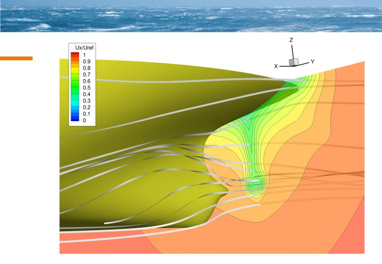
streamlines around the stern and the axial velocity field in the wake.
