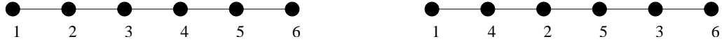
Fig. 4.2.1 Left: lexicographic ordering of grid points – Right: red-black ordering of grid points
