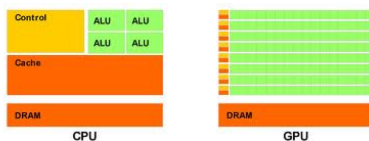
Figure 2: Design of a CPU and a GPU [9].
