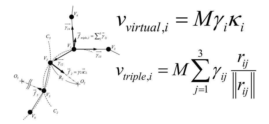
Vertex method based on Minimization of Grain Boundary Energy (1/2)
