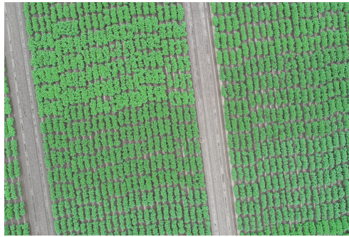
Figure 9: A 5472 \times 3648 image corresponding to the 2019-06-12 orthophoto in the time-series. Captured by the DJI Phantom 4 Pro at an altitude of 30 meters.
