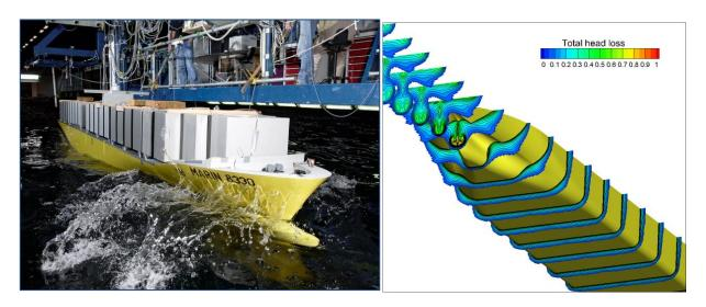
**Project Background** One of the most effective ways to reduce fuel consumption of a ship is to improve the hull form design. Computational Fluid Dynamics (CFD) plays an ever-increasing role to achieve this, as it permits extensive design studies prior to any model testing. Instead of using one CFD-computation, automatic optimization procedures can be used to evaluate a series of hull forms.
