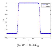
Figure 4.13: Results (two points per element) using two Legendre polynomials (up to order K = 1) for the advection equation with discontinuous initial condition, using  $\Delta x = 0.01$ ,  $\Delta t = 0.001$  and t = 0.25.
