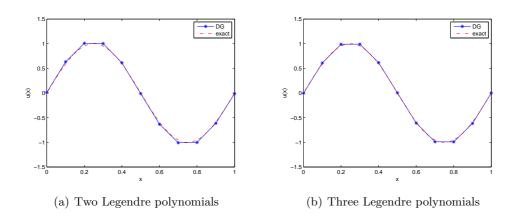
Figure 4.9: Results (one point per element) for the advection equation after t=2 with ten elements ( $\Delta x=0.1$ ) and  $\Delta t=0.001$ .
