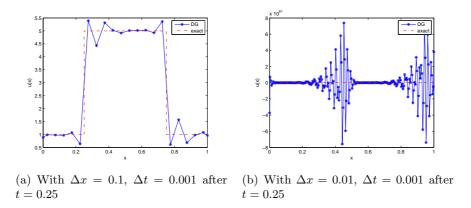
Figure 4.11: Results (two points per element) using five Legendre polynomials for the advection equation with discontinuous initial condition.
