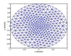
Figure 4.2: A coarse triangular grid using 576 triangles.
