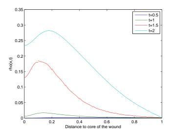
Figure 4.16: Vessel density with element size  $\Delta x = 0.1$  and time step  $\Delta t = 10^{-4}$ .
