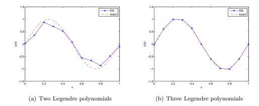
Figure 4.8: Results (two points per element) for the advection equation after t=2 with five elements ( $\Delta x=0.2$ ) and  $\Delta t=0.001$ .
