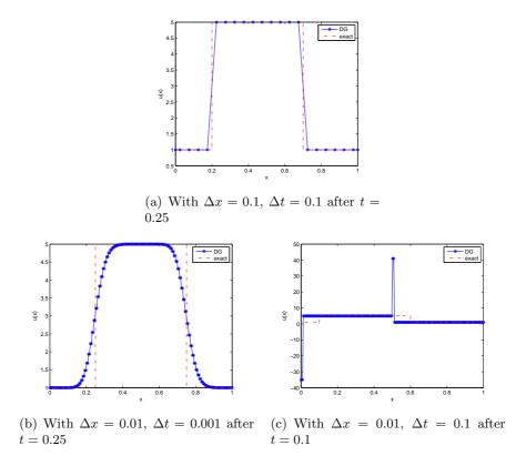
Figure 4.10: Results (two points per element) using one Legendre polynomial for the advection equation with discontinuous initial condition.
