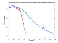
Choice for  $\omega_j$ :  $\diamond$  minimise  $||\mathbf{r}_i||$  w.r.t.  $\omega_j$  $\diamond$  Chebyshev nodes for f = 19 Hz
