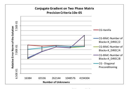
Figure 64: Relative Error Norm of the Solution  $\frac{\|X_{exact} - X_k\|_2}{\|X_{exact}\|_2}$  across various sizes for different variants
