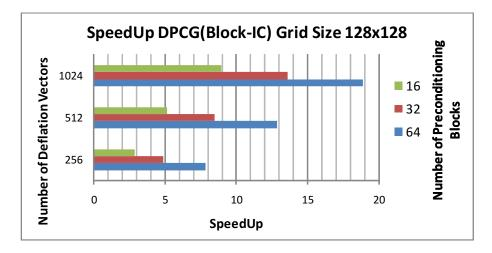
Figure 21: Deflated Block-IC Preconditioned Conjugate Gradient (Simple CUDA kernel) $\tilde{1}6k$ unknowns
