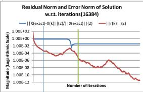
Figure 62: Conjugate Gradient with Block-IC Preconditioning for Two-Phase Matrix (Grid Size  $128 \times 128$ )
