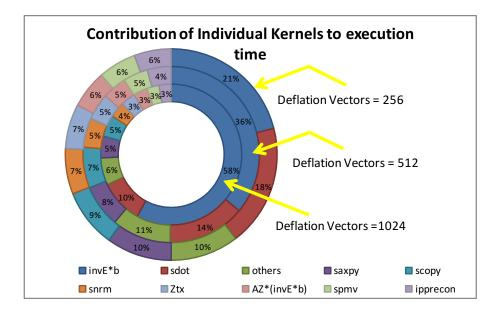
Figure 44: Deflated IP Preconditioned Conjugate Gradient. Grid Size  $(128 \times 128)$
