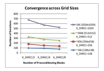
Figure 13: Decreasing iterations across block sizes (CG with Block-IC Preconditioning)
