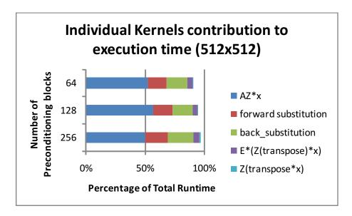
Figure 25: Conjugate Gradient with Deflation and Block-IC Preconditioning (Simple Version) Deflation Vectors=1024
