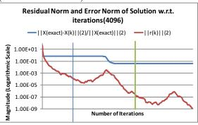
Figure 56: Conjugate Gradient with Diagonal Preconditioning for Two-Phase Matrix (Grid Size  $64 \times 64$ )
