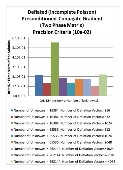
Figure 67: Two Phase Matrix with Density Contrast (100 : 1). Relative Error Norm of the Solution  $\frac{\|X_{exact} - X_k\|}{\|X_{\iota}\|}$
