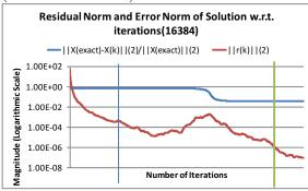
Figure 57: Conjugate Gradient with Diagonal Preconditioning for Two-Phase Matrix (Grid Size  $128 \times 128$ )
