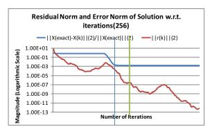
Figure 54: Conjugate Gradient with Diagonal Preconditioning for Two-Phase Matrix (Grid Size  $16 \times 16$ )
