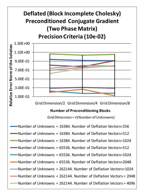
Figure 65: Two Phase Matrix with Density Contrast (10 : 1). Relative Error Norm of the Solution,  $\frac{\|X_{exact} - X_k\|_2}{\|X_k\|_2}$
