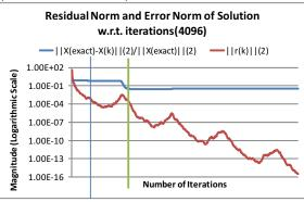
Figure 61: Conjugate Gradient with Block-IC Preconditioning for Two-Phase Matrix (Grid Size  $64 \times 64$ )
