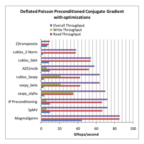
Figure 69: Bandwidth Break-Up. Grid Size (512 × 512). Number of Deflation Vectors = 4096. Optimizations applied to AZ storage and calculation.  $E^{-1}b$  calculation optimized with MAGMA Library. Grouping optimizations in Saxpy operations.
