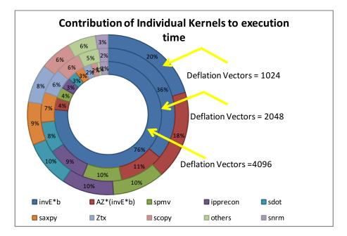
Figure 46: Deflated IP Preconditioned Conjugate Gradient. Grid Size $(512 \times 512)$
