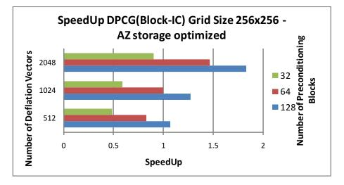
Figure 29: Deflated Conjugate Gradient with Block-IC Preconditioning.  $256 \times 256$  grid.
