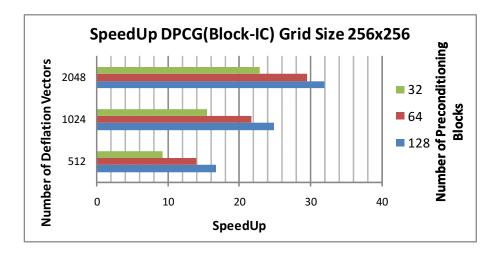
Figure 22: Deflated Block-IC Preconditioned Conjugate Gradient (Simple CUDA kernel)  $\tilde{6}5k$  unknowns
