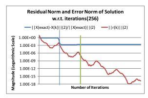
Figure 59: Conjugate Gradient with Block-IC Preconditioning for Two-Phase Matrix (Grid Size  $16 \times 16$ )
