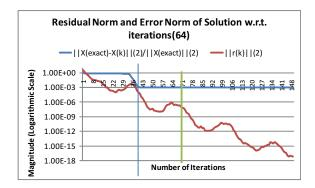
Figure 53: Conjugate Gradient with Diagonal Preconditioning for Two-Phase Matrix (Grid Size  $8 \times 8$ )
