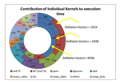
Figure 52: Deflated Preconditioned Conjugate Gradient. (AZ storage optimized and Magma BLAS based gemv) Grid Size  $(512 \times 512)$
