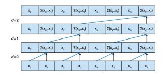
Figure 7: An Illustration of the Up-Sweep, or Reduce, Phase of a Work-Efficient Sum Scan Algorithm
