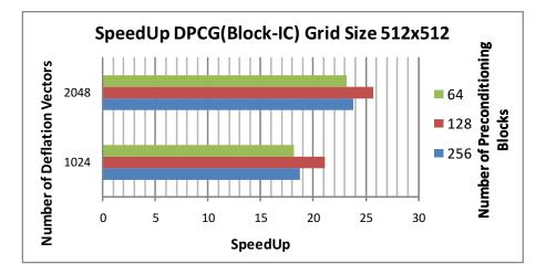
Figure 23: Deflated Block-IC Preconditioned Conjugate Gradient (Simple CUDA kernel) $\tilde{2}60k$ unknowns
