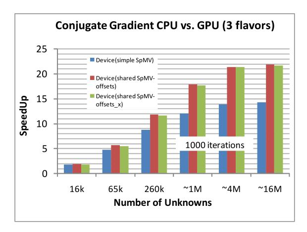
Figure 10: Conjugate Gradient on Host vs Device
