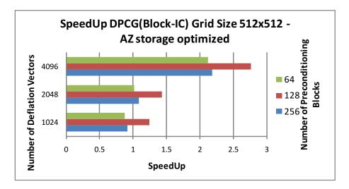
Figure 30: Deflated Conjugate Gradient with Block-IC Preconditioning.  $512 \times 512$  grid.
