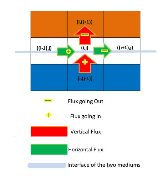
Figure 2: Flux entering and leaving a discretized cell
