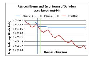
Figure 58: Conjugate Gradient with Block-IC Preconditioning for Two-Phase Matrix (Grid Size  $8 \times 8$ )
