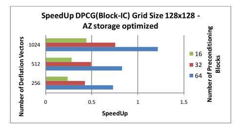
Figure 28: Deflated Conjugate Gradient with Block-IC Preconditioning.  $128 \times 128$  grid.
