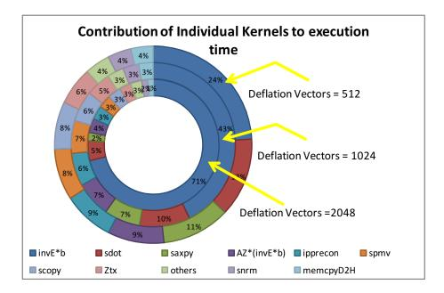
Figure 45: Deflated IP Preconditioned Conjugate Gradient. Grid Size $(256 \times 256)$
