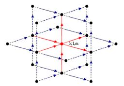
The red arrows represent the six unknown electric ded components lying on the edges and surrounding grid node  $(x_k, y_l, z_m)$ . The 24 blue arrows are the electric ded components corresponding to neighboring grid nodes which are needed to compute the discretization of the curl operator lying on the same edges as the entries of  $E_{k,l,m}$ . All matrices and vectors of (5) are described in detail and can be found in Appendix (??).
