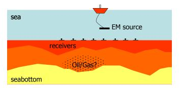
At the surface between sea and seabottom, a large number of receivers is placed. Next, a ship with a large cable, which *works* as an EM source, sails above the receivers.
