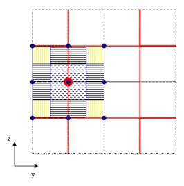
The figure shows the grid from besides, the x-direction is perpendicular to the paper. The blue dots represent the coarse grid electric field components,  $E_1$ , lying at the edges of the grid cells. The red dot in the middle represents the fine grid electric field component  $E_1$ . The thick red lines are the edges of the coarse grid cells, whereas the black lines represent the edges of the fine grid cells.
