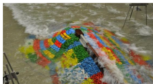
Figure 1 Example of obtaining wave field information near trunk of a breakwater
