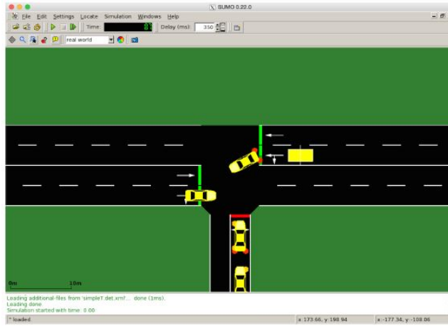
Figure 17: The T-junction considered here has ten links and three admissible traffic light configurations. The incoming lane from the South has four links: two going left and two going right. The other roads have three links each. The lane that crosses the junction has one link. The lane from which one can turn South has two links: one to cross the junction and one to turn South.
