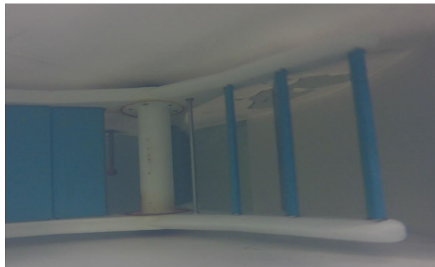
Figure 1.3: Snapshots reproduced from the testing of the OWM depicting the lamellas at the fully-open condition aligned with the flow
