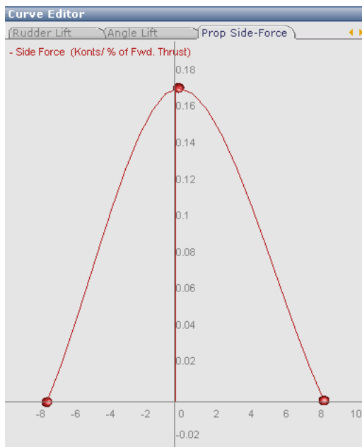
Figure 4.10: When the ships starts to accelerate, it banks over a bit and this is caused by a sideward directed force, also called the torque of the propeller. This force is not calculated in the ship editor, but read from this curve.
