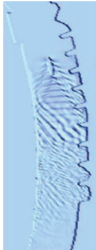
Figure 1. Wave pattern around a ship sailing through the river IJssel.
